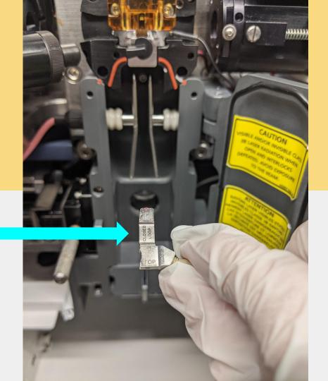
The Closed Loop Nozzle red o ring and label faces upwards when inserted into the Quartz Cuvette.
