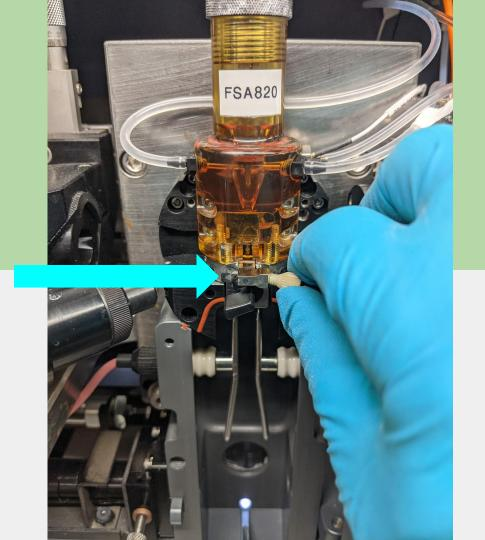
Turn the black knob clockwise to 12 o'clock to seat the red o ring up against the Quart Cuvette.
