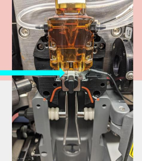
To remove the ceramic nozzle, turn the black knob counter clockwise to 9 o'clock.
